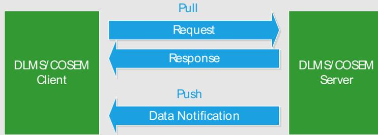
Figure 3 – Pull and Push operation
